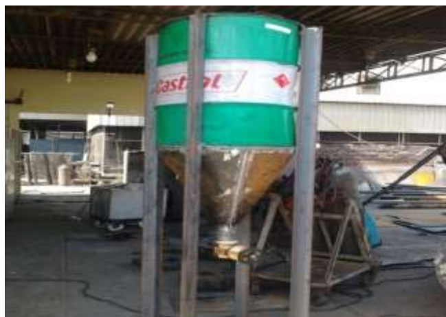
Figure 12 Centri-gravitational equipment under construction
